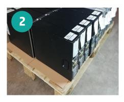
Make a layer by placing the desktop next to each other with the front facing the center of the pallet.
