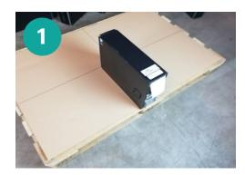
Define the center of the carton by drawing two lines, one crossing the other and place the desktops so they align from the center line towards the periphery of the pallet with the back side.
