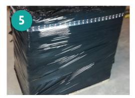
Isolate the pallet with black protective cover. Attach the KO-number on all sides.
