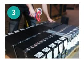
When the first layer is done, secure the desktops with tape and put a piece of carton on top.
